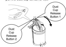
To empty the dust cup container, press on the trap door release button that is on the back side of the dust cup container.
